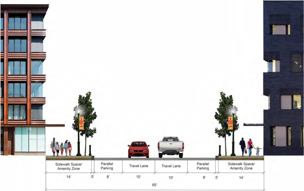
Figure 4.5.6 Conceptual Cross Section for a Local Access Street with On-Street Parallel Parking
