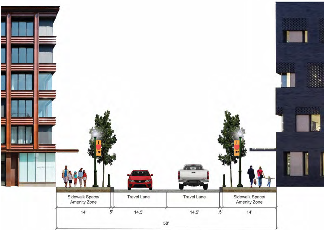
Figure 4.5.7 Conceptual Cross Section for a Local Access Street with No On-Street Parking
