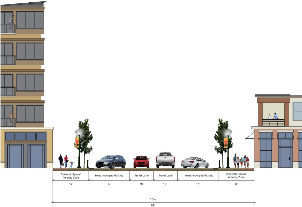
Figure 4.5.6 Conceptual Cross Section for a Festival Street with On-Street Angled Parking
