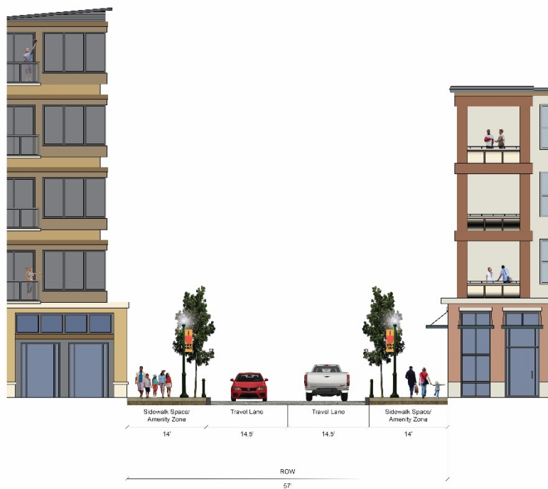
Figure 4.5.5 Conceptual Cross Section for a Local Access Street with No On-Street Parking
