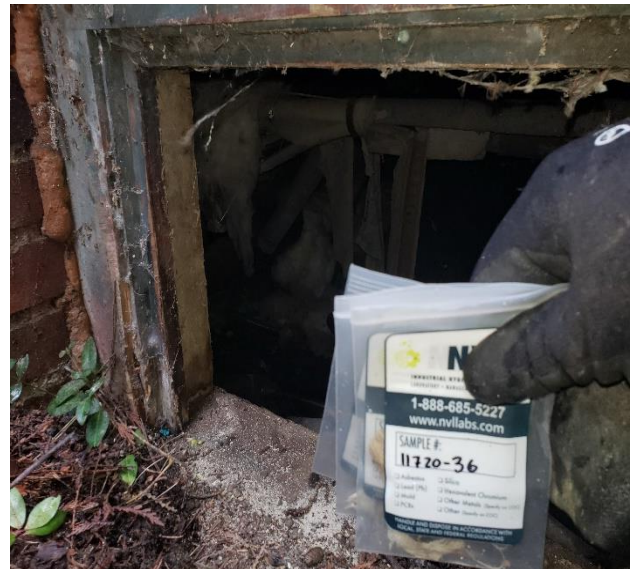
Photo #4: Sample 11720-36 through 38 & 60/60QA & 61: TSI (on 3" OD metal hot water piping). (44% Chrysotile) Location: Building 8 Crawl Space and East Garage Building
