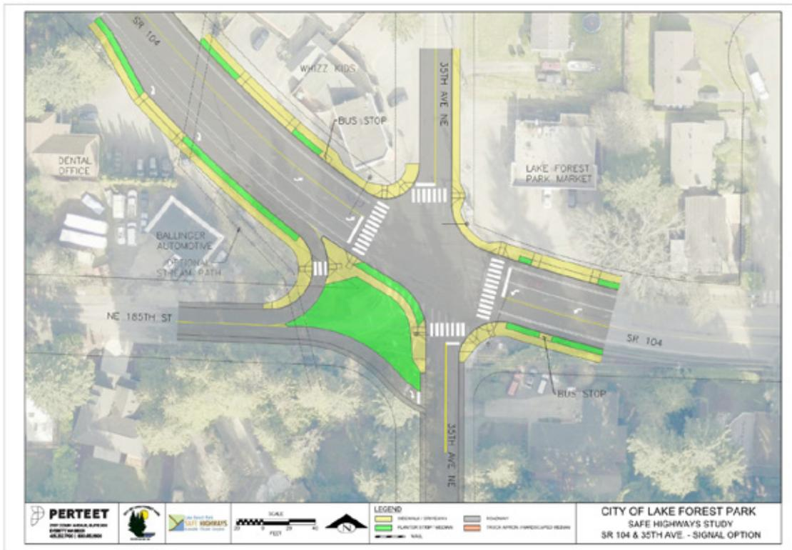
The improved signalization alternative eliminates direct access from NE 185<sup>th</sup> Street to create a four-legged intersection.
