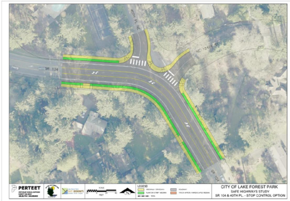
This Alternative considers more modest changes to the existing intersection, including more pronounced pedestrian crossings of 40<sup>th</sup> Place NE and NE 184<sup>th</sup> Street. This option does not provide a pedestrian crossing of SR 104.
