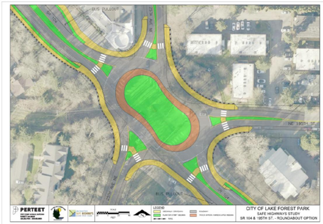
Roundabout alternative features more of a peanut shape to accommodate the five legs and geometrics of the connecting roads.
