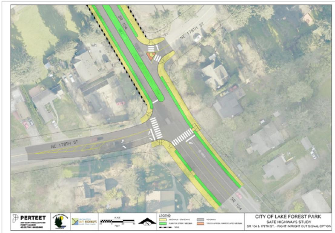
This option signalizes the west leg of NE 178<sup>th</sup> Street and makes the east leg right-in/right-out only.
