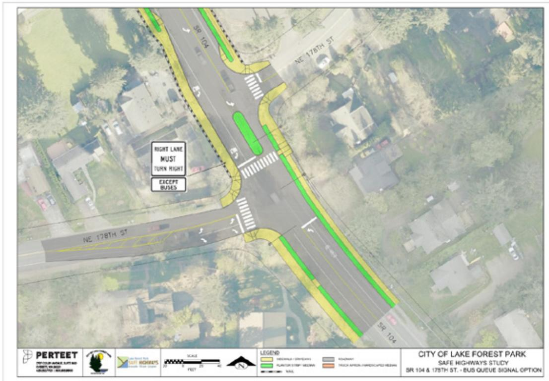
This option signalizes the west leg of NE 178<sup>th</sup> Street, retains left-in access to the east leg, and provides a southbound right-turn lane that can also serve as transit queue jump.
