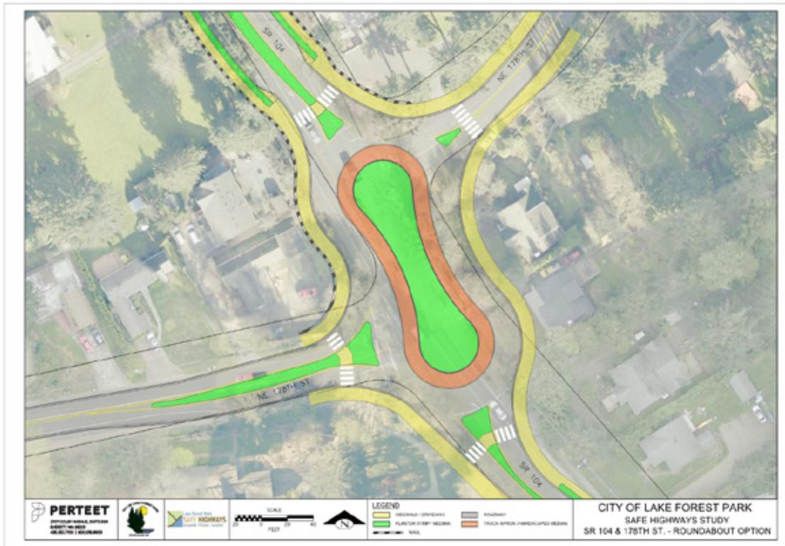
Figure 5. An oblong, peanut shaped roundabout could accommodate demands at the NE 178<sup>th</sup> Street intersection during most of the day, but not the peak hours.
