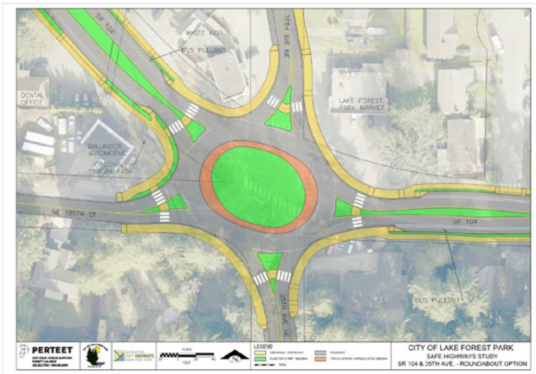
The roundabout alternative includes a large footprint and oblong shape to accommodate access to all five legs of the existing intersection.
