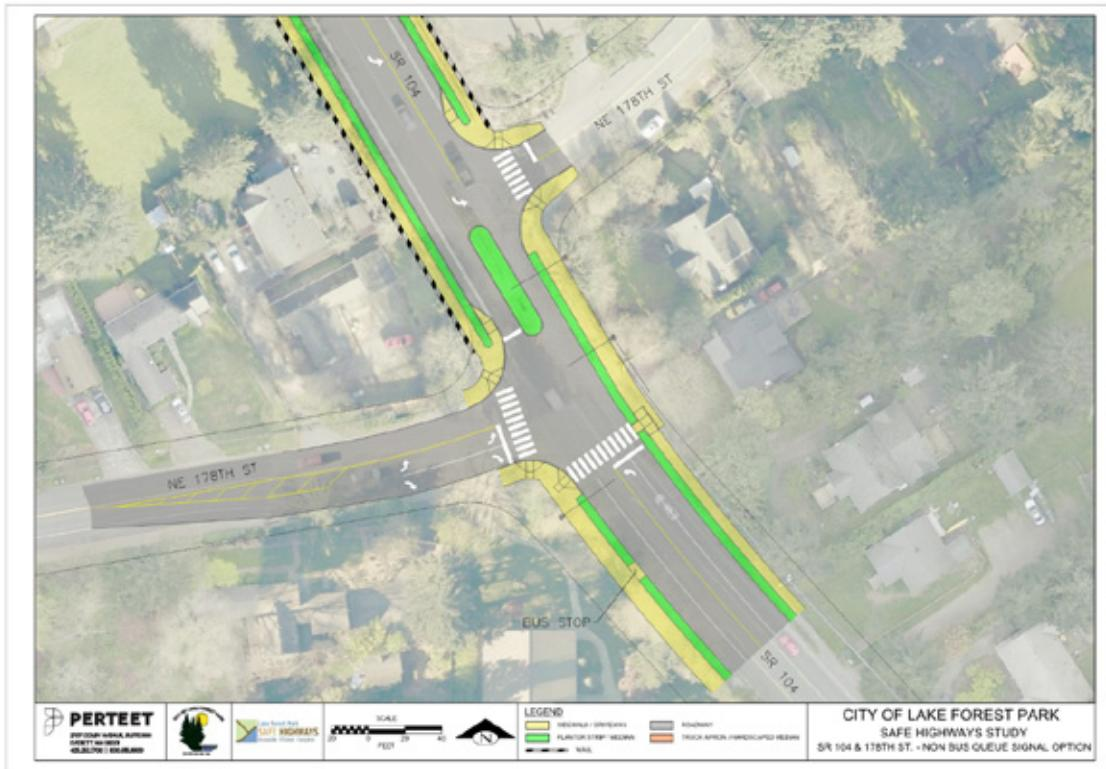
This option signalizes the west leg of NE 178<sup>th</sup> Street and retains left-in access to the east leg.
