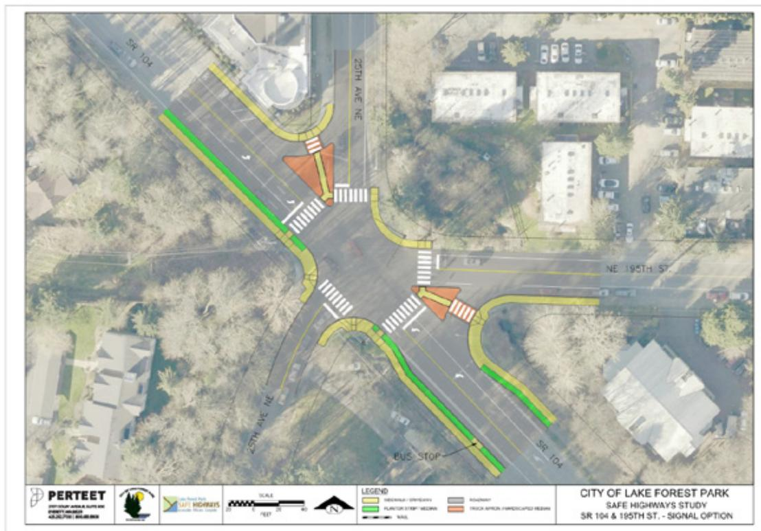
The improved signalized option makes the intersection more compact and realigns pedestrian crossings.
